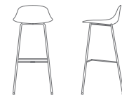
282-STL Jump Bar Height Mini Stool H38 W17.25 D18.75 SEAT H30.5 W18 D16 FOOTREST FROM SEAT H18
