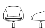
292ST Martini Plus height adjustable swivel H31.75-34.5 W28 D28 SEAT H17.5-20.5 W21 D20 BASE DIAMETER 28
