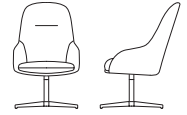
293FH Martini lounge high back swivel base H41 w26.5 d32 SEAT H17.5 w21 d20 BASE DIAMETER 33
