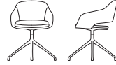
290H4/291H4 Martini high four swivel base H31.25 w23 d23.5 SEAT H19 w19 d18 BASE DIAMETER 26.25
