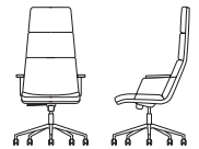
845 crisscross high back swivel H51-54 w26 d29 SEAT H17-20 w21 d18.5 ARM H 25.5-28.5 BASE DIAMETER 29
